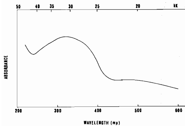
Figure 7. Electronic absorption spectrum (reflectance), molar absorbance on arbitrary scale, of \text{Ni}(\text{P}^n\text{Bu}_3)_4 at 15^\circ\text{C}
